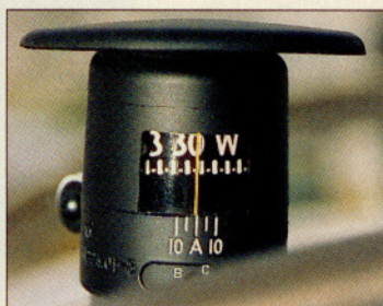
Zlinware includes an airspeed indicator that makes two trips around the dial, two mag compasses, and a gauge that tells of spar cracks.
