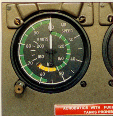
Zlinware includes an airspeed indicator that makes two trips around the dial, two mag compasses, and a gauge that tells of spar cracks.
